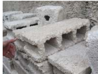
Poor Quality Concrete blocks with broken edges and not cured properly
