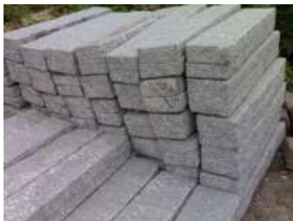
Properly shaped stones with straight edges
