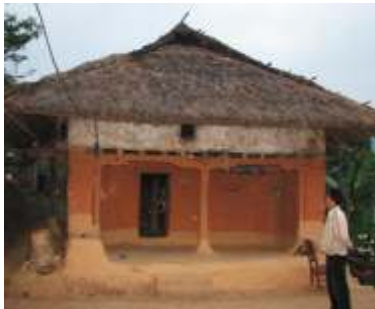
Adobe walls with thatch hipped roof - Sikkim
