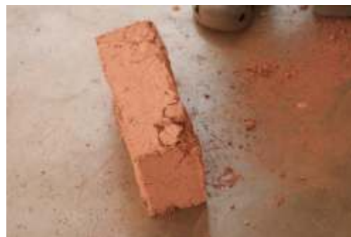
Uneven edges and poor quality brick
