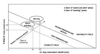
Figure 2. Schematic diagram that can be used to issue warning of rainfall-induced landslides based on rainfall threshold.
