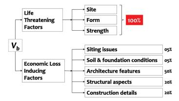
Figure 2.4: Flowchart for Vulnerability Estimation of a Building (values of Economic Loss Inducing Factors are given alongside the flowchart [ (Murty, Raghukanth, et al. 2012)]
