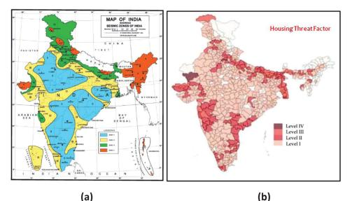
Figure 2.1: (a) Seismic Hazard Map [ (IS 1893(Part 1) 2016)], and (b) Housing Threat Factor [ (Ramancharla and Murty 2014)]
