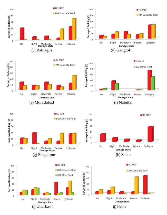
Figure 5.2: Possible Damage States of building typologies in the cities in seismic Zone IV cities with highest EDRI
