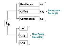
Figure 2.3: Flowchart for Exposure Estimation of a Building (values of Importance Factor I recommended in IS1893 (1) are given in brackets)
