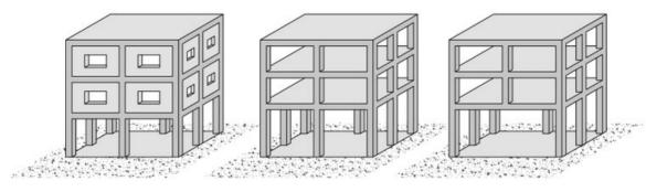
(a) Stiff and strong upper floors due to masonry infills (b) The columns in one storey longer than those above (c) Soft storey caused by discontinuous column
