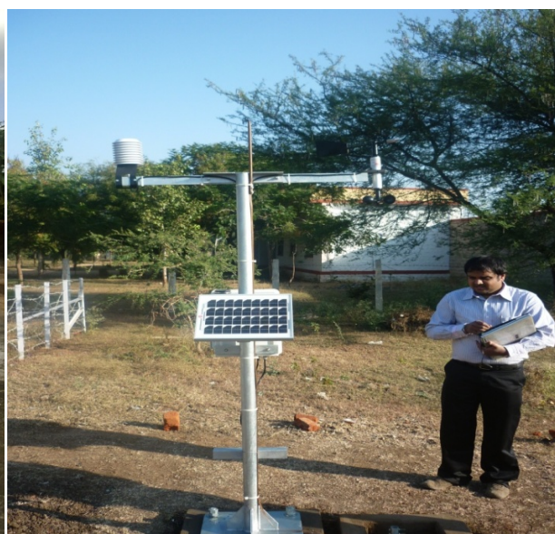
GPRS enabled Solar Power Telemetric Weather Station
