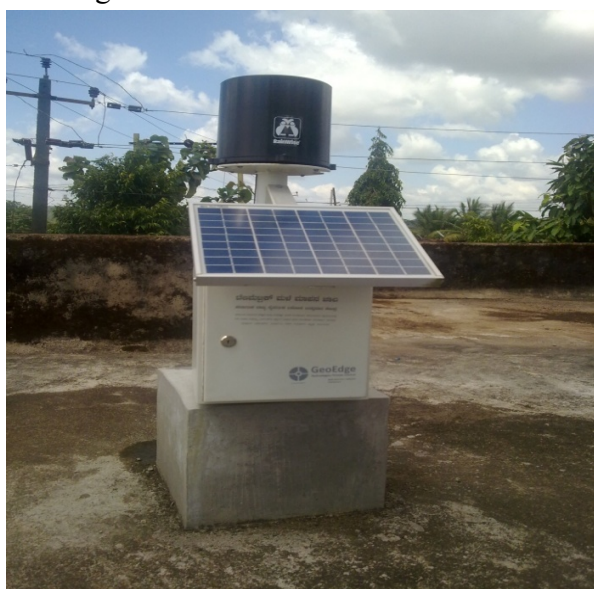
GPRS enabled Solar Power Telemetric Rain Gauge
