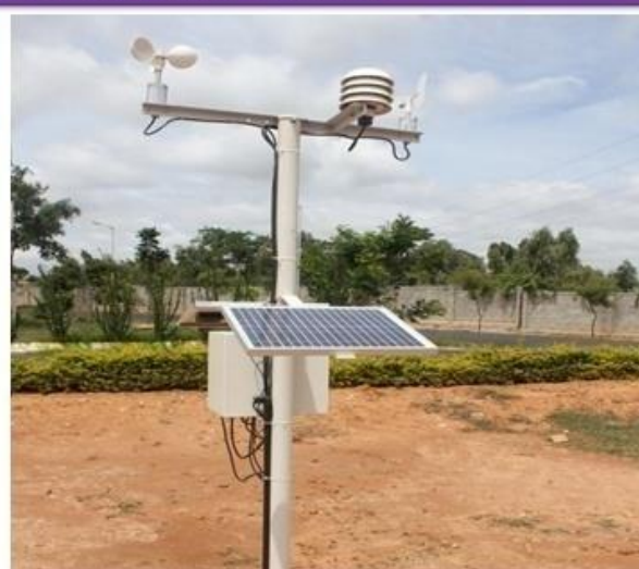
GPRS enabled and Solar Powered Weather Monitoring Station at every ~ 250 sq. Km
