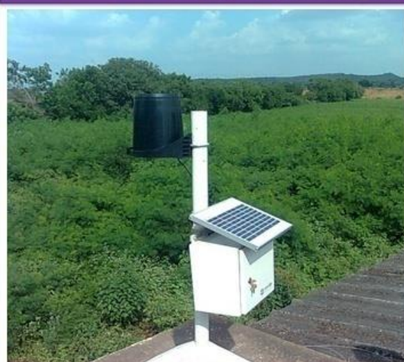
GPRS enabled and Solar Powered Telemetric Rain Gauge (TRG) at every ~25 sq. Km
